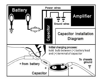
**Note:** Capacitors are most effective when there is a 18" (0.5m) or less of wire between the cap and the amplifier(s).
